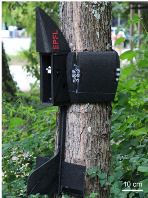
Fig. 3 | PercHug robot perching vertically on a tree by hugging. Replicated from Askari et al. 7 .
